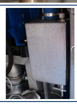
The water lock has two functions. Mainly it separates the air/water mixtures that is pumped into the water lock from the vacuum pump.
