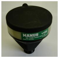
The VRM module is a valve. The module works together with the Sentry unit. When the pressure is too low in the vacuum system. This VRM (valve) is opened and air can flow in into the vacuum system till it reaches its desired value. Together with the Sentry unit it ensures that the vacuum level is stable and not too low.
