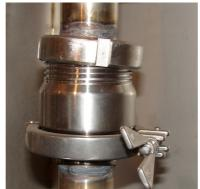
Ensures that no air can return into the air separator.
