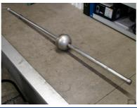
The floater is mounted on a vertical guiding bar placed inside the center of the air separator. Inside this bar are 4 electronic contacts points. (HLH, HLL, ML, LL) These contacts are triggered when the floater (magnets inside the floater ball) moves past them. These signals are used to operate the COSMO VMI and the MAGYAR air separator. For a detailed explanation of the working and operating principle of these contacts see "working principle COSMO VMI".
