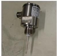
The air bubble sensor detects when air is entering the air separator and regulates the milk pump speed.
