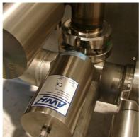
Milk valve opens when milk is being collected and measured. This milk valve is opened pneumatically. The milk valve closes when the tank is unloaded at the milk factory. It is placed after the meter in the down-tube. By closing this valve the milk cannot return into the measuring system when the milk is unloaded.
