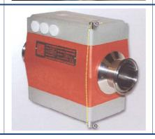
The COSMO VMI is fitted with an electric magnetic induction meter (MID). The central measuring element of the MID is a stainless steel measuring tube positioned in a magnetic field of coils. When milk or any other conductive fluid flows through the tube it generates a  $% \left\{ \left( 1\right) \right\} =\left\{ \left( 1\right) \right\}$ voltage proportional to its velocity or flow. This results are transmitted as a digital output signal for a further processing system.
