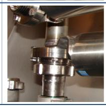
The vacuum valve is closed to maintain a vacuum after the vacuum pump has stopped.
