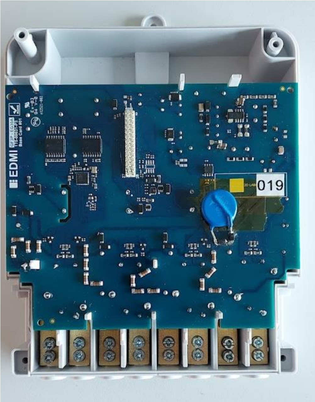
Inside- PCB bottom board
