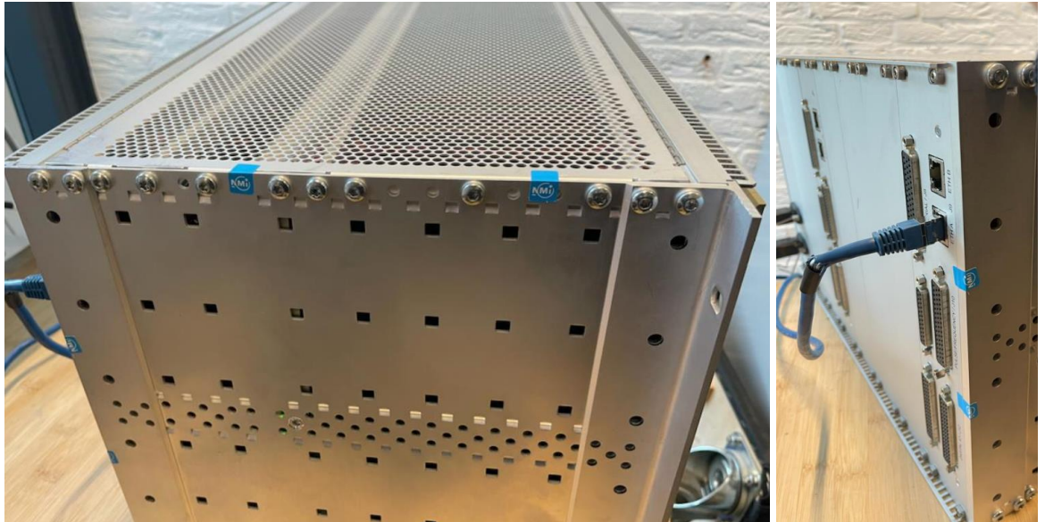
Figure 8 Example sealing of Sigma 3 against opening using sticker seals from back and sides.
