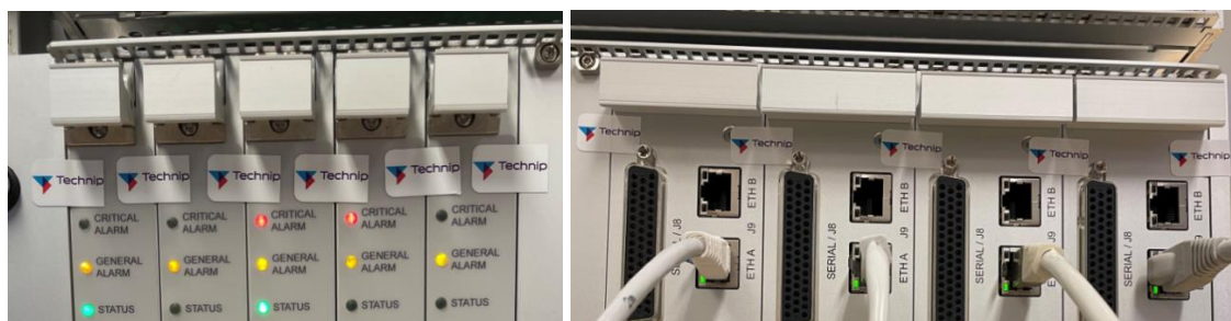
Figure 7 Example of sealing of Expansion IO PCA front side (left); back side (Right).
