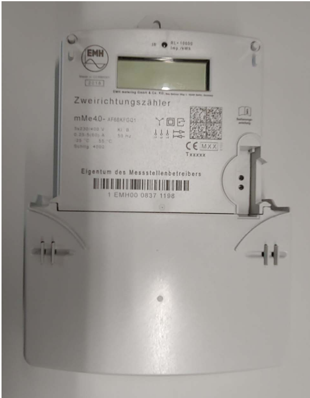
Housing with Terminal Cover
